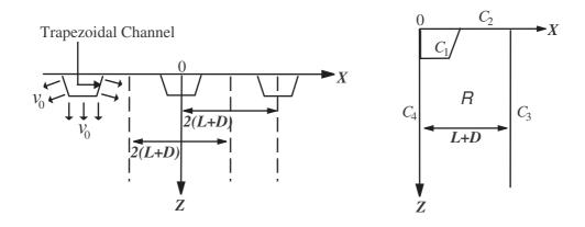
Figure 1: Geometry of periodic trapezoidal channels
