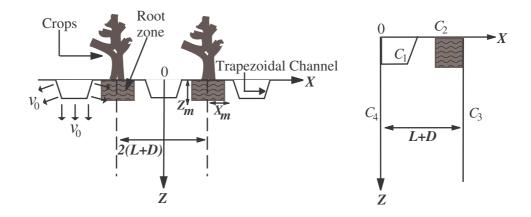
Figure 1: Geometry of periodic trapezoidal channels with roots zone
